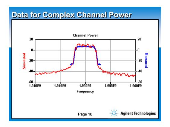
This shows data for both the simulated (virtual) test and the measured (actual) test.
