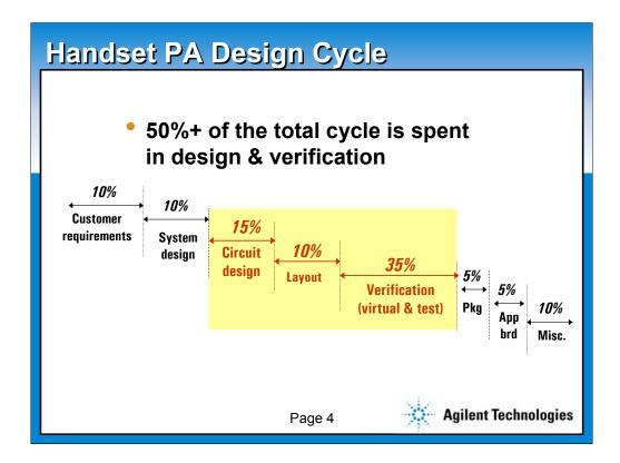
These numbers are based on the experience of the Agilent Solution Services consulting team; they've charted the design cycle for a number of RFIC companies, and this is consistent overall. The integrated Simulation and Measurement system targets the largest piece of this cycle: the verification segment.
