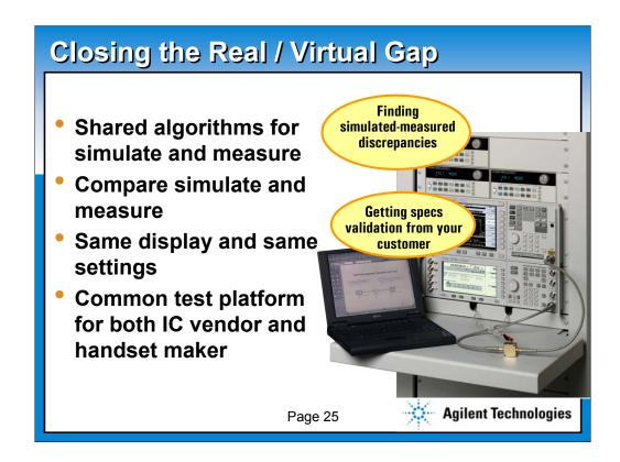
The ValiFire system validates the algorithms used in both simulation and measurement. It provides standard displays and charts both simulated and measured data and compares them to the specification. By automating data taking, ambiguity on measurement technique is eliminated leading to much quicker correlation between the chip maker and their customer the handset designer.
