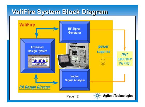
PA Design Director is the system "wrapper" software that integrates the ADS modules and the test equipment included with the system. Refer to the product overview literature for more specifics on what's included. To summarize here:
