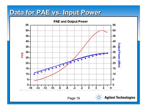
This shows both the power output and the Power Added Efficiency (PAE) vs. the input power for both a simulated (virtual) test and the actual test. The same scale on the left is in two units: % for PAE and dBm for power output. You can read the corresponding power input on the bottom scale.
