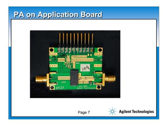
This is the 3G amplifier on its application board that we tested for most of this presentation. It is encapsulated in a plastic package and, in this phase of the design, the output matching network is placed on the PC board.
