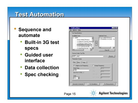
The above is the software front panel for the Design Director. It sets up a test schematic within ADS and switches between Simulated and Measured with the push of a single button
